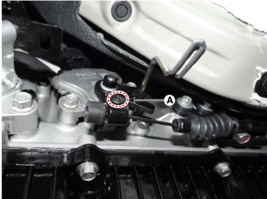
2. Remove the parking release cable from the bracket after loosening a bolt (A).
